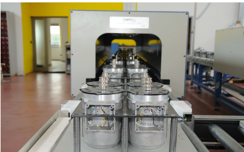
TUNNEL OVEN: By infrared lamps to have the pre-heating and the first gelification. the resin.
